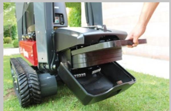
Stabilization plates holder with locker
