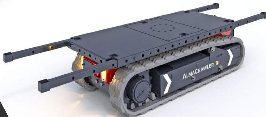
Four support beams on each angle provide added support for extra-large loads. Can be positioned into place manually extending the platform either longitudinally or laterally.
